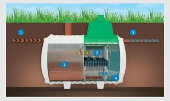
Tricel Novo wastewater treatment plant has an overall efficiency of 95.9% BOD removal
