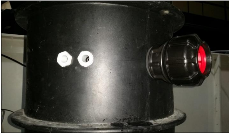
Figure 13 Cable Glands and Outlet connection fitted.
