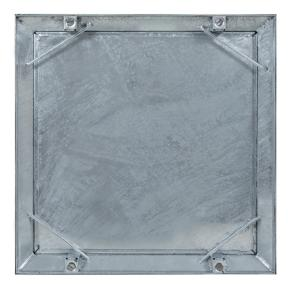
This range of recessed covers is designed to be in-filled with a suitable screed or concrete, and are available in a range of clear opening sizes and feature, as standard, four locking screws and rubber neoprene seal to resist gas egress and water ingress. Gas and airtight under normal atmospheric conditions – suitable for internal applications.
