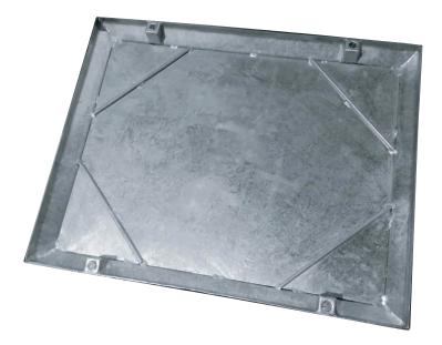
This range of recessed covers is designed to be in-filled with a suitable screed or concrete, and are available in a range of clear opening sizes and feature, as standard, four locking screws and rubber neoprene seal to resist gas egress and water ingress. Gas and airtight under normal atmospheric conditions – suitable for internal applications.
