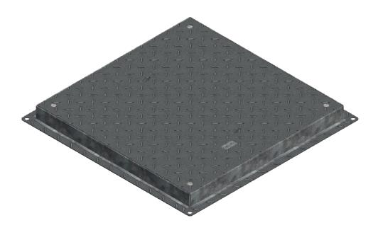
Suitable for small vehicles up to 15kN (1.5 tonne) wheel loads, 5 tonne gross vehicle weight, with speeds under 20 mph. This includes domestic driveways and very light industrial areas, where small trolleys and private cars/vans can manoeuvre, such as trolley parks and hospital wards.
