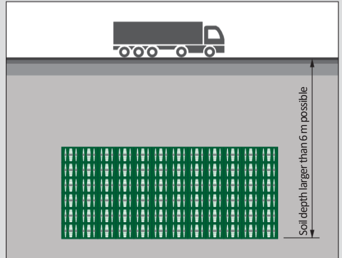
High installation depth of a multiple-layer storage/infiltration system
