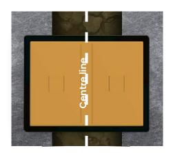
Always position the trench cover board **centrally** over the trench as illustrated.
