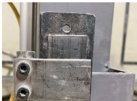
Image showing deflection across 800mm gap at 6mm with 800kg pressure
