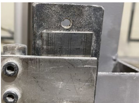
Image showing deflection across 800mm gap at 4mm with 400kg pressure
